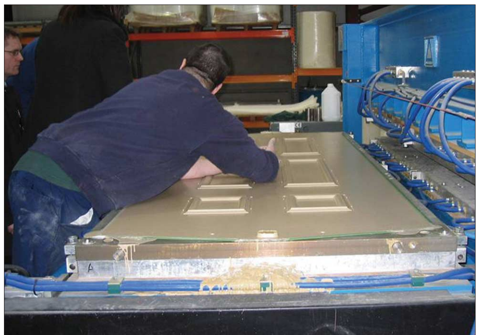
A GRP door skin under production at New World Developments.
