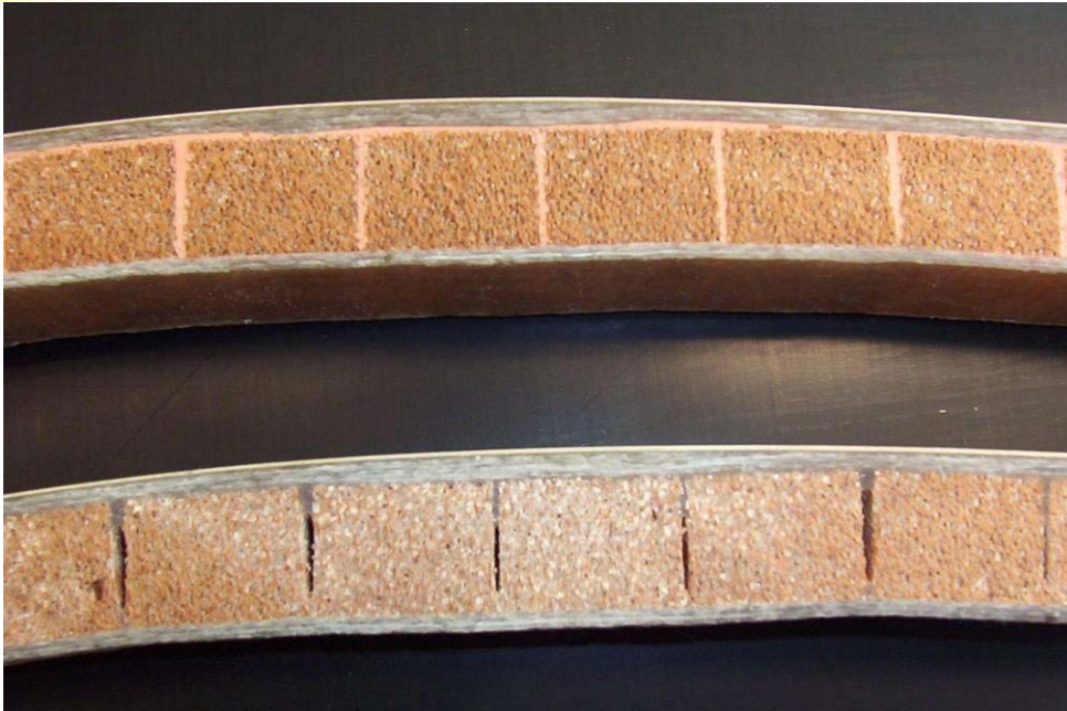
Crystic Crestomer 1196PA bonding PVC cored laminate.
