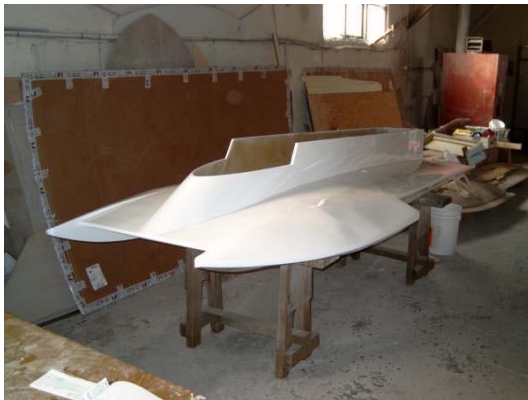
The Crystic LS 88PA gelcoat surface finish is enhanced by using Crystic Crestacoat 5000PA barriercoat and Crystic VE 679PA skincoat, which reduces cracking and provides a long term high quality gelcoat surface.
