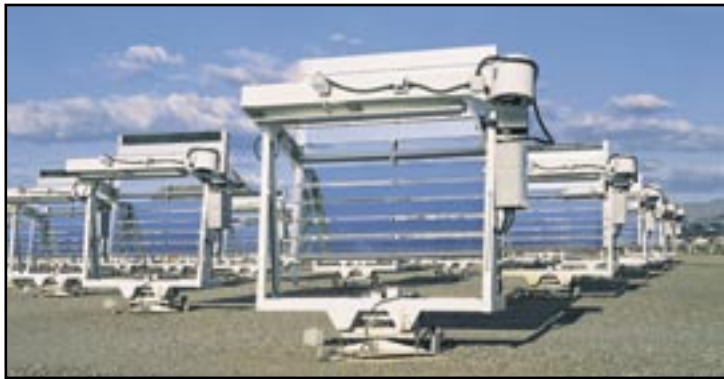
Extreme natural exposure conditions accelerate product weathering, two to three times faster than normal locations.
