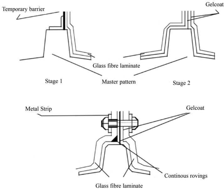
150mm or so, to hold the two halves of the mould together.
