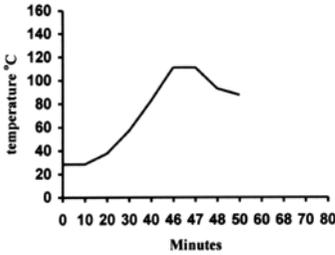
Figure 16 - Equivalent post curing times and temperatures.
