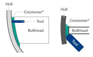
Ensure that the Crestomer® fillet at least touches the line mentioned in Step 2 (A). If the fillet is short of the line, a larger fillet tool is required (B). If the line cannot be seen, a smaller fillet tool can be used (C). The working time available for steps 6 – 9 using Crestomer® 1152PA is 50 minutes at 25°C using 2% medium reactivity MEKP.
