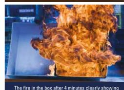
The fire in the box after 4 minutes clearly showing the protective properties of Crystic Fireguard Topcoat 75PA Excel on the left hand side
