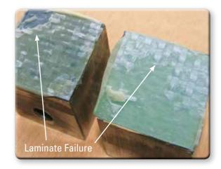
Result of GC 252PA adhesion test showing that failure is internal within
