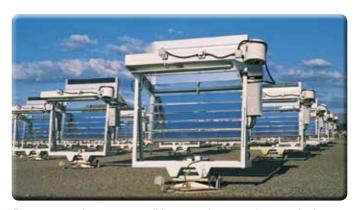
Extreme natural exposure conditions accelerate product weathering, two to three times faster than normal locations.
