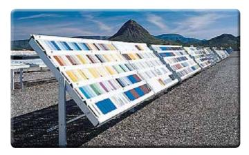
Extreme natural exposure conditions accelerate product weathering, two to three times faster than normal locations.
